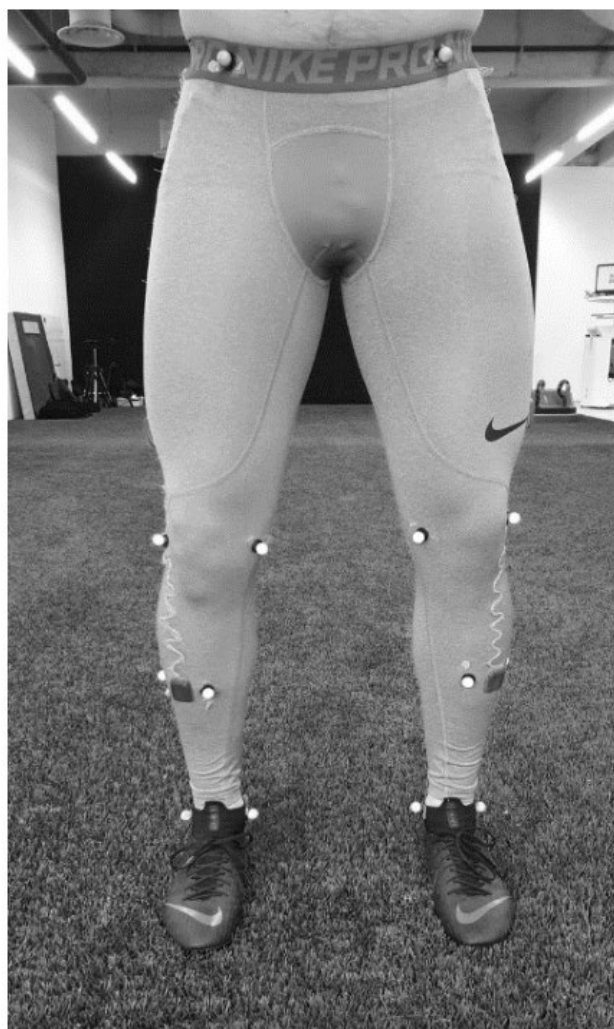
Figure 5. Prototype 1. Sensors are the black square units connected to the wiring; the white spheres are reflectors of the VICON system
